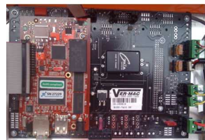
Buff 7400 Motherboard for PCMS-548, 320, 320X, 1232 & 1500C
